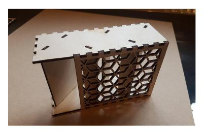
2) Lay down one of the side panels and glue in angled panels as shown below
