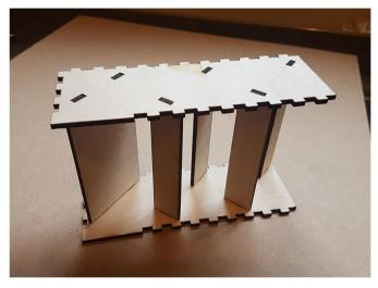
6) Glue on base panel. Elastic bands can be used to hold the tower in place while drying.
