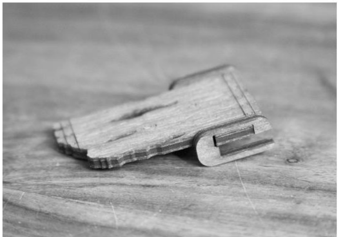
23) Assemble the plank as shown above, apply glue to both side clips, ensure they are facing the right directions (towards the deck) before gluing in place.
