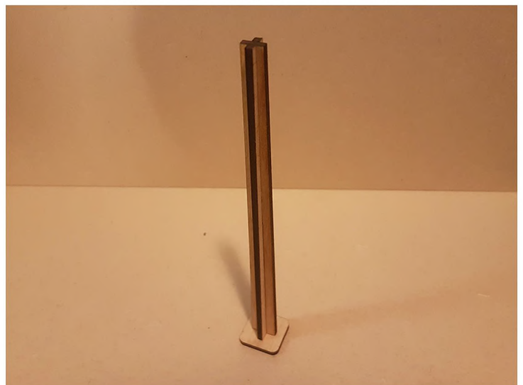
Apply glue to the inside edges of both vertical sections and slid them together. Then glue them down into the magnet base (magnets facing downwards).
